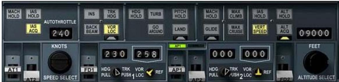
adjust CRS as required to centre deviation needle
